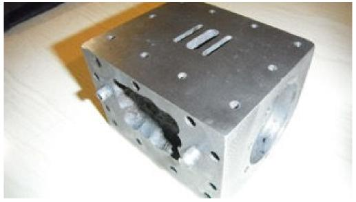
Brent Coburn is in the middle of a tear-down inspection of his NZR Super "Q" loco which is 40 years old. The boiler needs to be re-certified as well. He showed one of the cylinders which has pitting on the slide valve surface but the bore has been honed and is in good condition.
