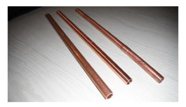
finish and cut cleanly. The tubing needs to be turned down to obtain satisfactory ligaments on the tube plates and clearance around the 32 tubes involved.
